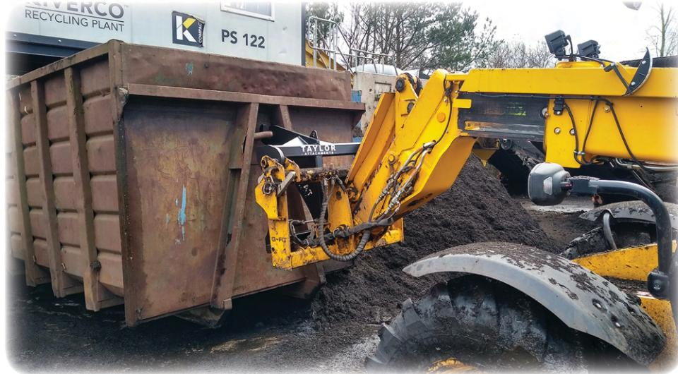
Commonly used in green waste and recycling industries for a speedy and safe way of moving empty 'roll on-roll off' skips. We've been told these save huge amounts of time and costs compared to using the lorries to manoeuvre the skips.
