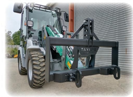
Expertly designed to float when in use to reduce rubber wear on your scraper.
