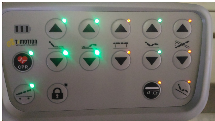
Mattress platform height lock, will lock Reverse Trendelenburg, Trendelenburg and Auto-Chair too.
