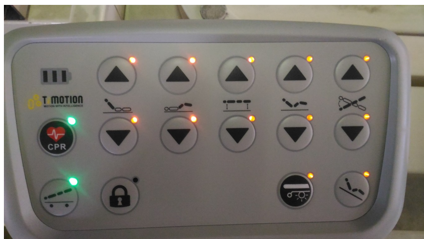
When total lock of the movements (press Function Lockout + Auto-Chair) is activated, CPR and TRENDELENBURG movements will work for Emergencies (Under bed light will work as well).
