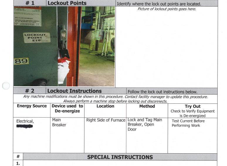
Reference: Typical minimal lockout procedure – 29 CFR 1910.147 App. A
