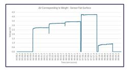
Capacitance (t∝RC) Measurement with 1MΩ resistor
