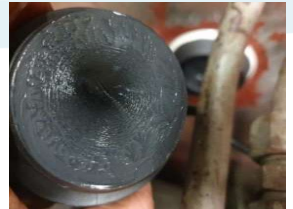
A fresh layer of coupling agent providing optimal sound transmission
