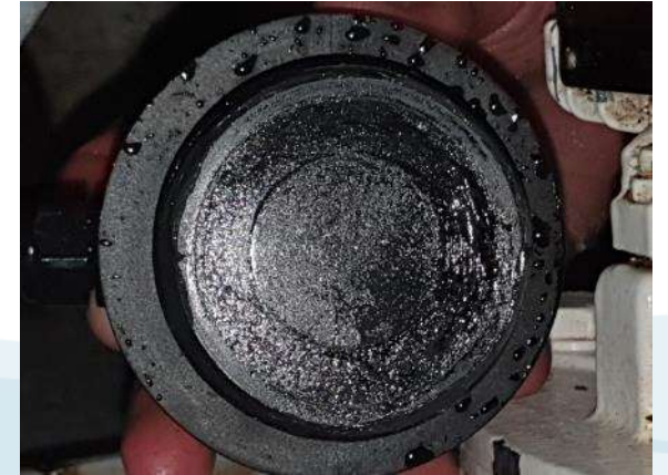
Dried out coupling agent reducing sound transmission
