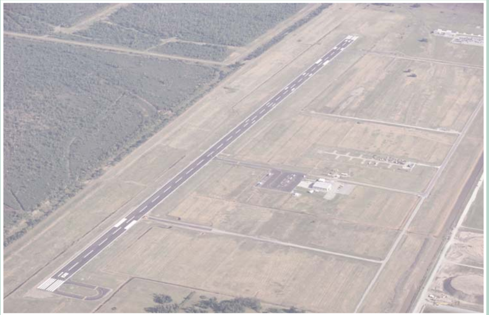
Pictured is an aerial shot of the South Lafourche Airport's new improved runway. The runway is 6,500 feet long and can accommodate larger aircrafts weighing up to 75,000 pounds.
