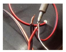
$\underline{\textbf{NOTE: isolate and secure the connection}} \text{ . Make sure the wires will not in contact with the back of the loudspeaker surf}$
