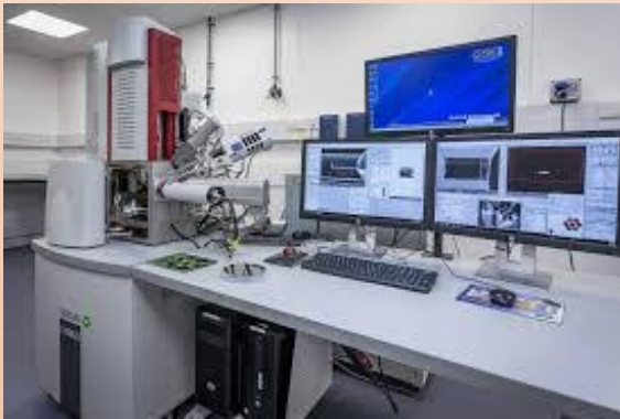
TESCAN LYRA 3 equipped by EDX, EBSD, FIB
