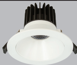
Small Design Standard Kit, 9.5W, 900lm, CRI90, Ø72-82mm cut out, 50° beam, IP65, IC-4, c/w dimmable flicker-free driver. R730 W3KV2 (3000K, White)
