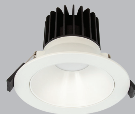
Medium Design Standard Kit, 12W, 950lm, CRI90, 100-110mm cut out, 90° beam, IP54, IC-4, c/w dimmable flicker-free driver. R611 W3K (3000K, White)
