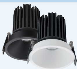
Titian 8W Recessed Fixed LED Spotlight IP54; 230V; 8W; 3K; 38°. A171WH/8W/3K/38° White A171BK/8W/3K/38° Black
