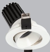
Design Standard Tilt Kit, 9.5W, 900lm, CRI90, 85-92mm cut out, 32° tilt, 50° beam, IP54, IC-4, c/w dimmable flicker-free driver. R750 W3K2 (3000K, White)
