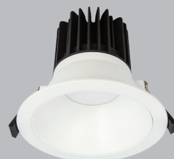
Medium Design Standard Kit, 12W, 950lm, CRI90, 100-110mm cut out, 90° beam, IP54, IC-4, c/w dimmable flicker-free driver. R611 W3K (3000K, White)
