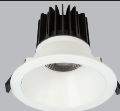
Medium Design Standard Kit, 12W, 1000lm, CRI90, 100-110mm cut out, 50° beam, IP54, IC-4, c/w dimmable flicker-free driver. R610 W3K (3000K, White)
