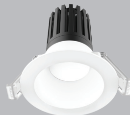
Exterior Small Design Standard Kit, 9.5W, 870lm, CRI90, Ø72-82mm cut out, 50° beam, IP65, IC-4, c/w dimmable flicker-free driver. R730 XW3KV2 (3000K, White, 316 STS)
