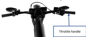
Before each use, check that the throttle handle rotates properly and ensure that it returns to its original position when rotated to prevent accidents.
