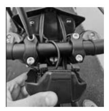
Please, frequently check that the screws holding the handlebars on the bar mounts are tight.
