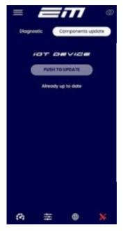
This screen is used to update the IOT device with new features or fix any problems.
