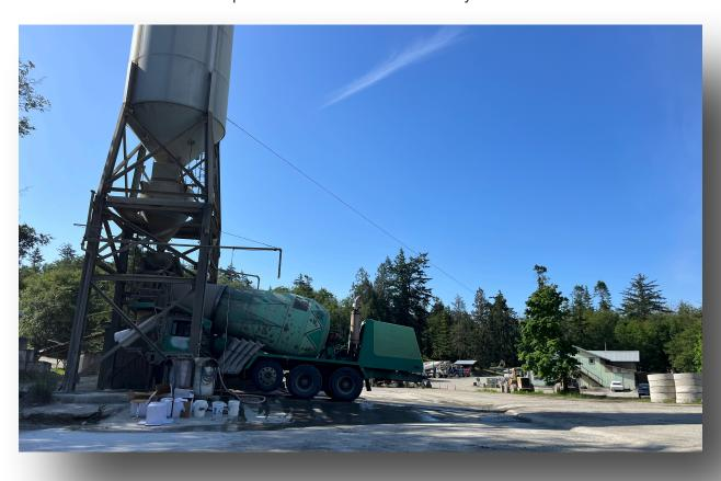
E5 can be added on site but this may result in slump loss from the plant to the site. In any case, a qualified representative from Sustainable Structures LLC should be present or should have thoroughly trained the Ready Mix Provider so that dosing is done per E5 manufacturer recommendations. E5 has to be added after all other ingredients have been thoroughly wetted, this is crucial. Water can be added on site as necessary to maintain slump. All loads should be
