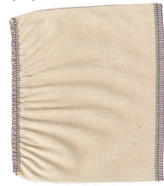
1. Place the tricot pieces right sides together. With the differential set at 1 (normal), stitch along the 6" side of the soft fabric together along one 6" edge, trimming about 1/4" off the edge. When sewing on very lightweight fabric, you may notice that you have a puckered edge.
