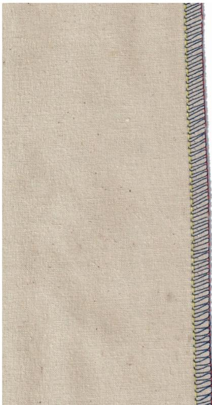
For this exercise, the overlocker will be threaded for a wide 3-thread overlock stitch using only the Left Needle and thread colors to match the color-coded threading path on the overlocker. Adjust all thread tension settings for a balanced stitch as indicated in chart below.
