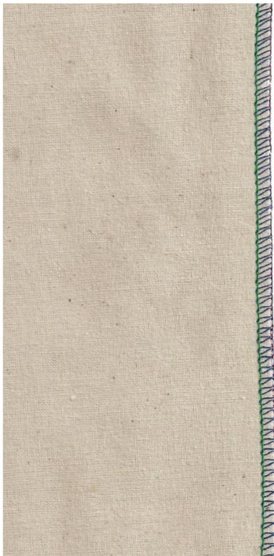
For this exercise, you will thread the overlocker for a 3-thread narrow overlock stitch using the Right Needle and thread colors to match the color-coded threading path on the overlocker. Adjust all thread tension settings for a balanced stitch as indicated below.
