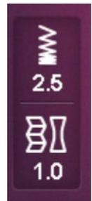
The settings for Stitch Length and Differential Feed can be adjusted using the Slider Control, or for fine adjustments using the <+> and <-> icons. In addition, from this screen you can launch an animation that illustrates the changes to the stitch as various adjustments are made. If a change has been made to the setting, the number will appear in yellow.
