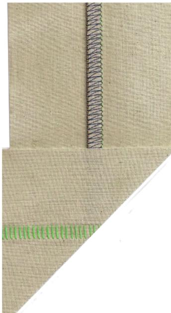
**Decorative Thread Tip:** A heavy thread such as Jeans Stitch or Pearl Crown Rayon can be used in the looper for a more decorative look. When working with heavy decorative threads, loosen the Upper Loper tension and lengthen the stitch length as needed for the desired look.
