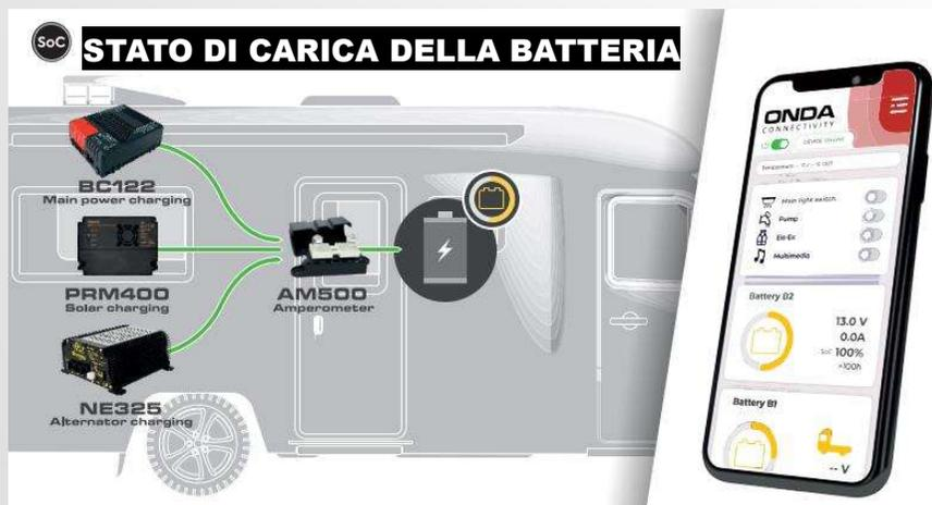
The diagram shows a side view of a camper van with three charging components: BC122 Main power charging, PRM400 Solar charging, and NE325 Alternator charging. These are connected to an AM500 Amperometer, which is connected to a battery. A smartphone displays the ONDA app interface, showing the battery status for Battery 02 (13.0 V, 0.0 A, 100% SoC) and Battery 01.
