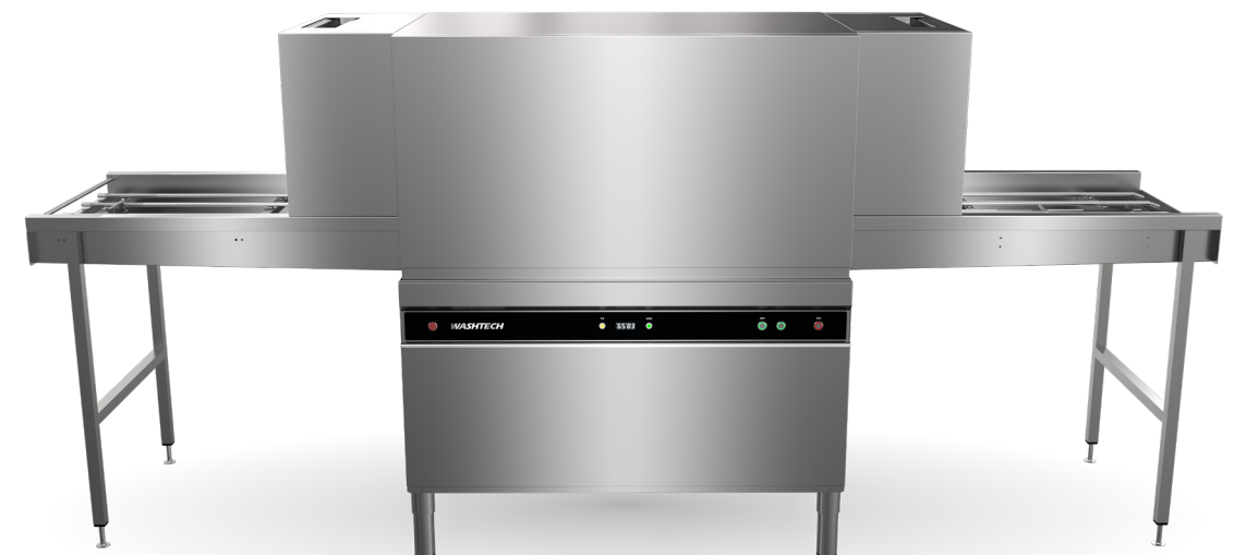
Image: CK100 c/w 620mm rack path, central pawl drive integrated inlet and outlet rail tables and 300mm vent hoods
