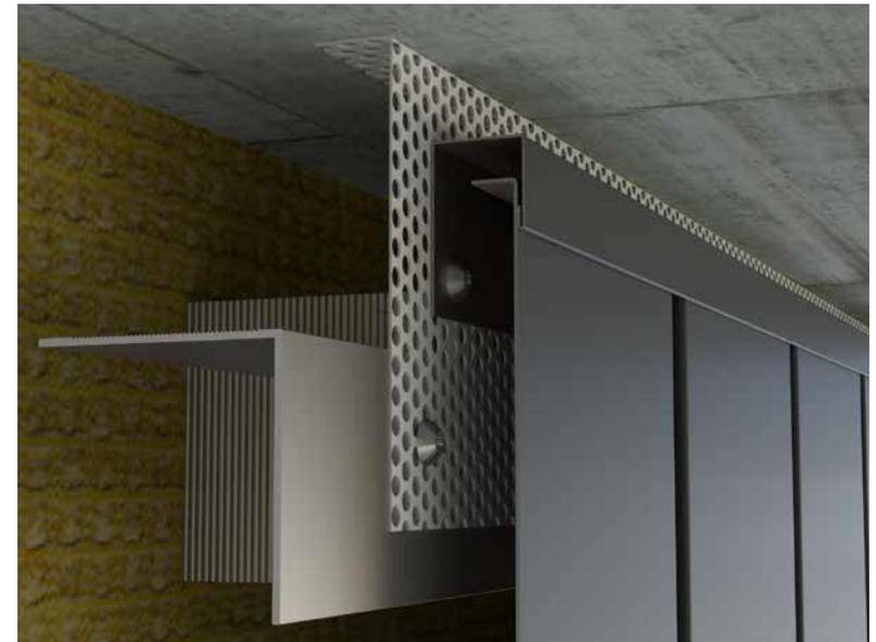
Figure 88 · Head detail vertical siding
