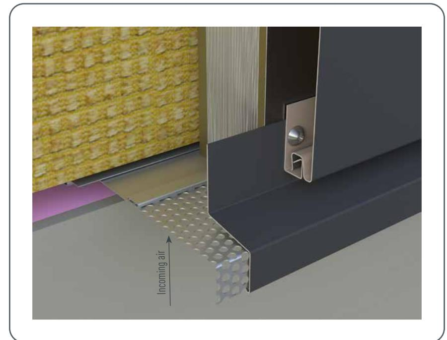
Figure 70 • Starter profile for horizontal installation
