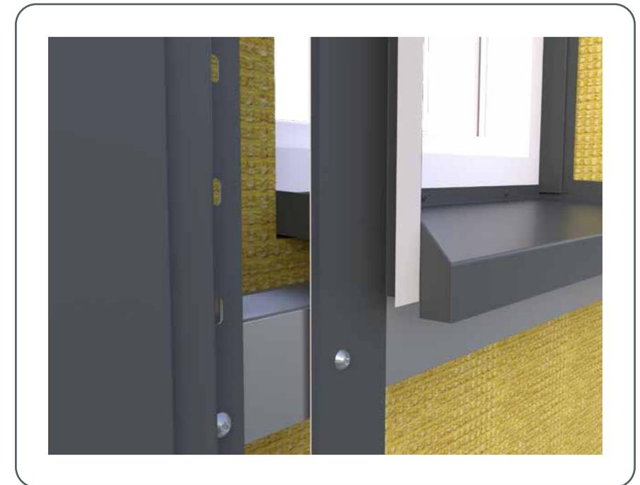
Figure 96 • Installation of pocket profile
