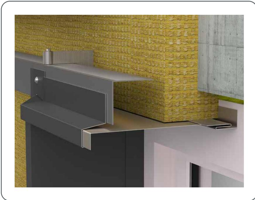
Figure 101 • Installation of drip edge
