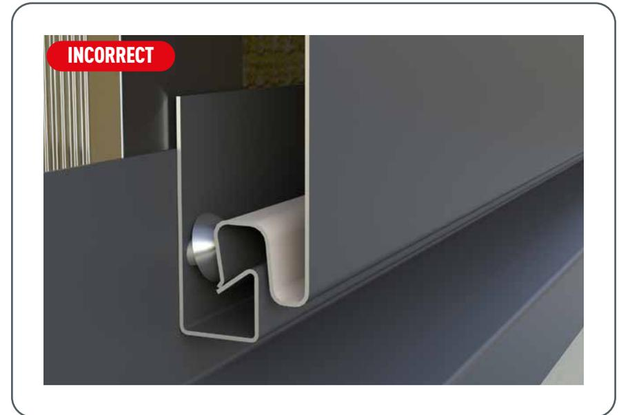
Figure 77 • Fastening misaligned starter profile
