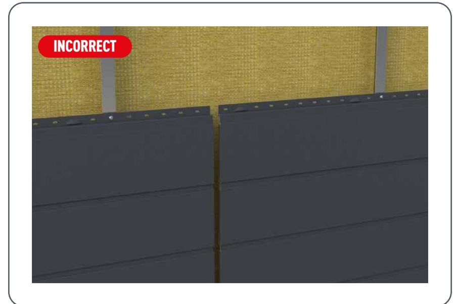
Figure 92 • Butt joint is not recommended
