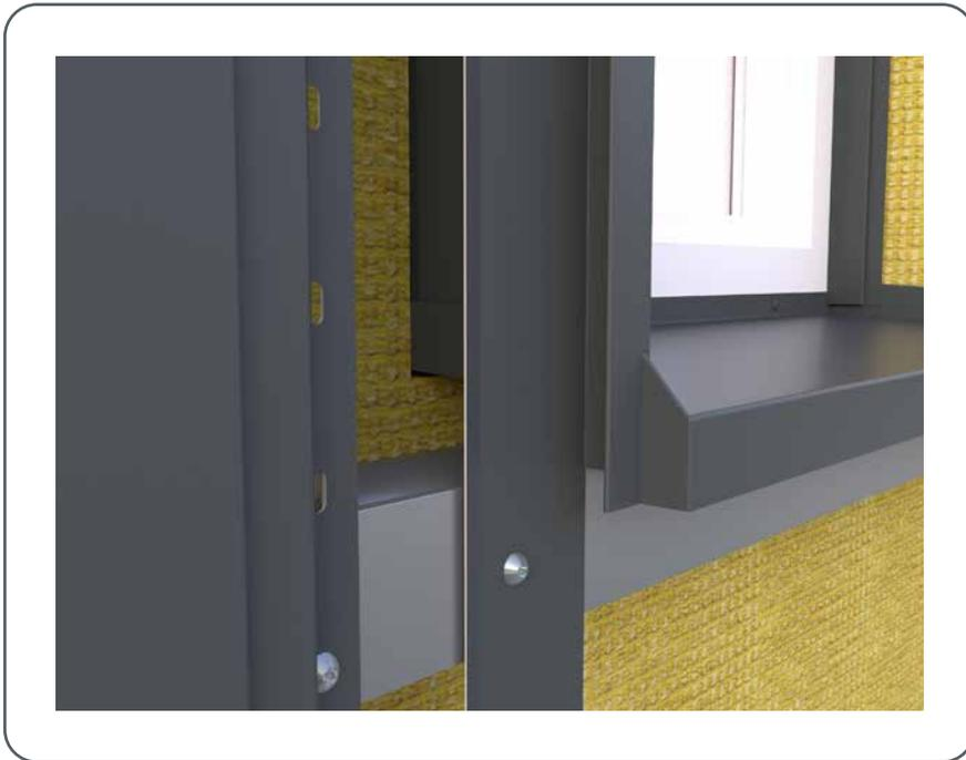
Figure 99 • Installation of jamb flashing
