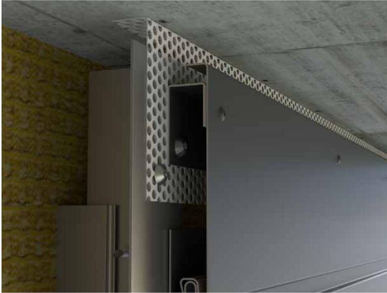
Figure 87 · Head detail horizontal siding
