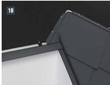
In most cases with roof sections with 29 × 29 or 44 × 44 rhomboid roof tiles, an eaves plate must be manufactured by the processor. Usually a roof step requires a bespoke starter flashing made by the installer himself. This means that you can easily start with a 29 × 29 or 44 × 44 rhomboid roof tile (Image 1A + 1B).
