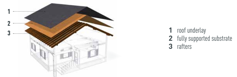
Figure 4 • Single-shell roof structure
