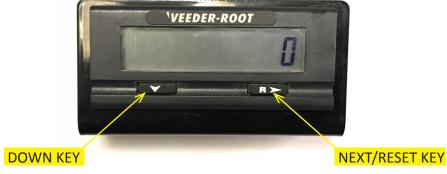
Programming parameters can be accessed by pressing the Down Key. To edit a parameter use the Down key to scroll until the desired parameter appears on the screen. Pressing the Next key will cause the leftmost digit of that value to begin to flash. Use the Next and Down keys in combination to choose individual digits and change their value.
