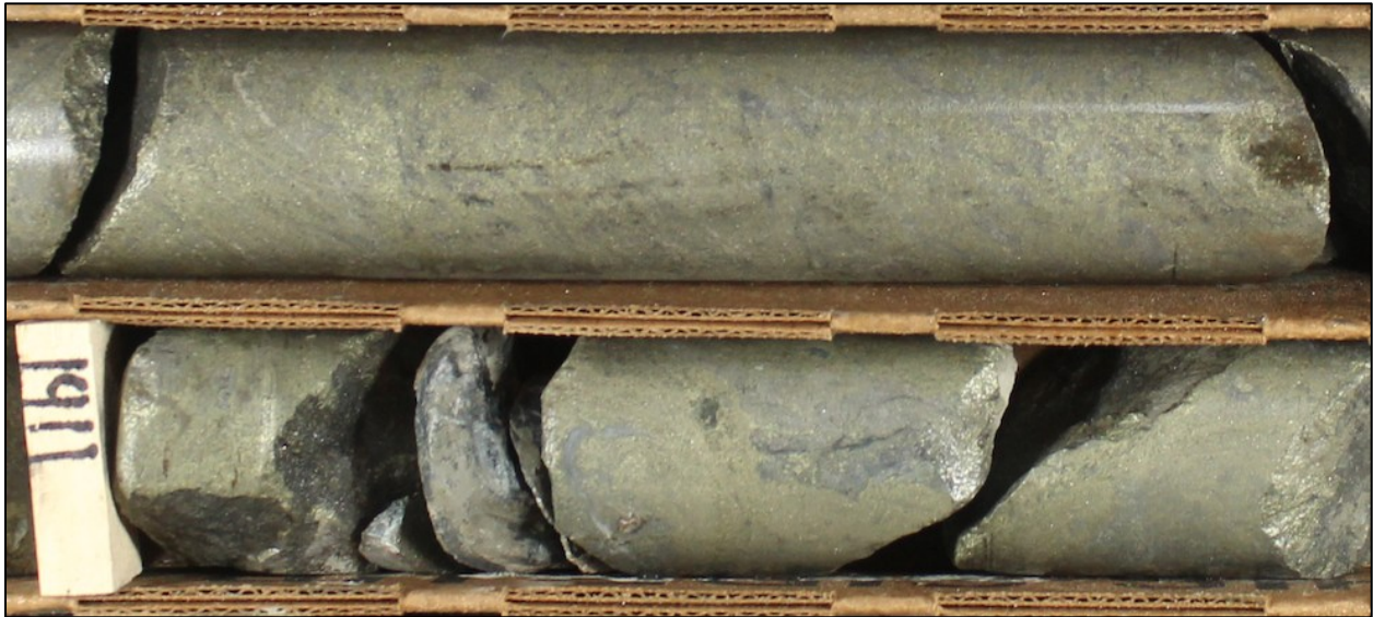
Figure 7.10: Massive Chalcopyrite in Drill Core From a 1.2-M Sample Grading 9.8% Cu, 6.1 g/t Au (Drill Hole KM-21-26, 581.6-582.8 M) (Smith, 2024)
