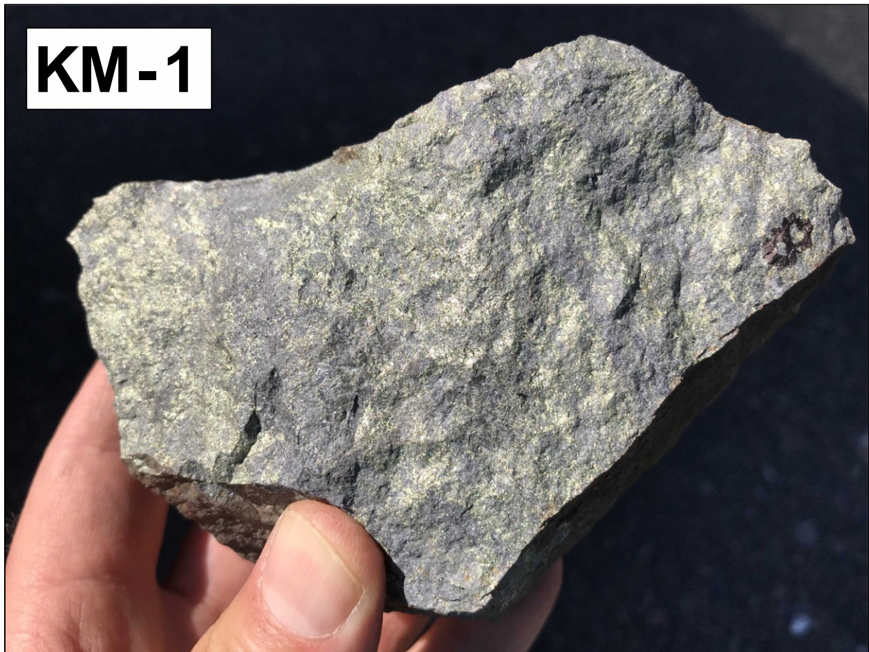
Figure 7.9: Massive Sulfide Mineralization Collected by Author on Mine Dump at No. 1 Shaft (Smith, 2024)
