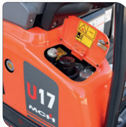
Rifornimento carburante Refueling
