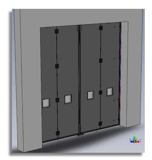
Door Engineering's Four-Fold 800, Tornado resistant door system, is the only Four-Fold door system available that has been designed for, tested and passed ICC-500 & FEMA 361 storm shelter requirements.
