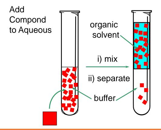
Measure analyte in aqueous phase before and after shaking with organic solvent.
