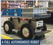
Full autonomous handling allows automatic parts delivery to assembly line, and material transfer between various locations.
