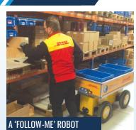
Utilizing 'follow-me' functionality, EffiBOT follows a picking operator and no cart is pulled or pushed manually, providing an obvious productivity gain.
