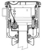
The A1004EVR-210, -215 Series include the features of the A1004-210, -215 Series as shown on pages 24-27. The EVR Series incorporate the 494118A Drain Assembly.
