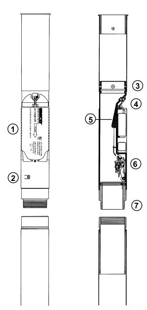
Provides tank with automatic fuel shutoff at 95% capacity
