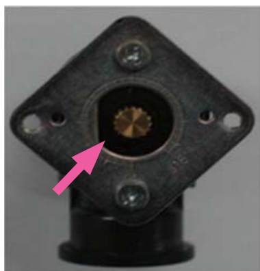
Turn the gear clockwise to open the valve manually
