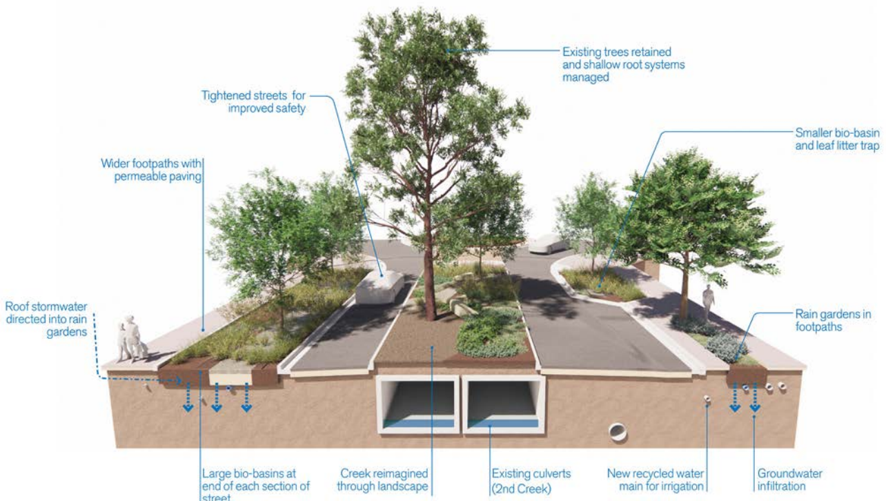
Figure 4. Water sensitive urban design schematic for St Peters Street upgrade. Graphics: by LANDSKÅP for the City of Norwood, Payneham and St Peters.
