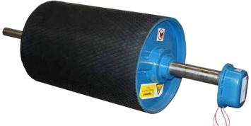
Ideal for the separation of larger or heavier ferrous metals. The extremely heavy-duty design suits difficult and arduous environments such as found in mining and recycling operations. The internal electromagnetic coils are mounted on thick shafts and revolve with the pulley to ensure that the conveyed product is exposed to the strong magnetic field at all times when energized.
