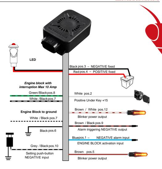
Refer to the "PIN to PIN Wiring List" for your specific vehicle model at this link: <a href="https://tech.patrolline.it/uploads/download/ListaCablaggi WiringList.pdf">https://tech.patrolline.it/uploads/download/ListaCablaggi WiringList.pdf</a>
