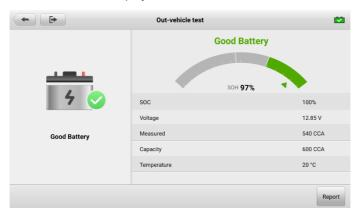
Figure 12-11 Out-vehicle Test Results Screen
