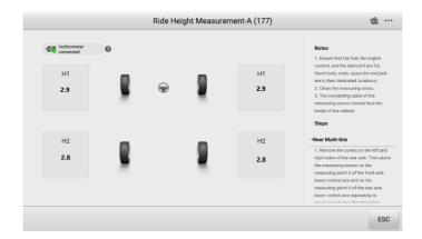
Figure 13-3 Ride Height Measurement Result Screen
