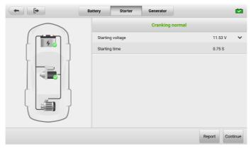
Figure 12-8 Starter Test Result Screen
