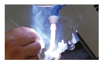
The use of laser technology permits precision parts, for example plastic injection molds, to be altered and repaired with an accuracy of up to .004 inch.
