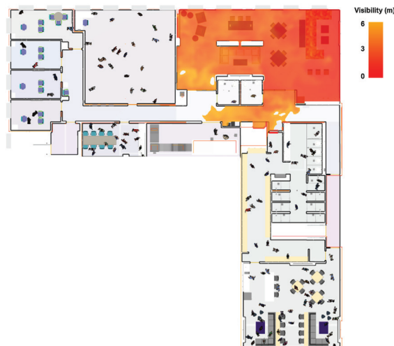
Fig. 8. Patten Gym, Northwestern University, Evanston, Ill. Smoke and egress modeling, 2020. Graphic by SmithGroup.
