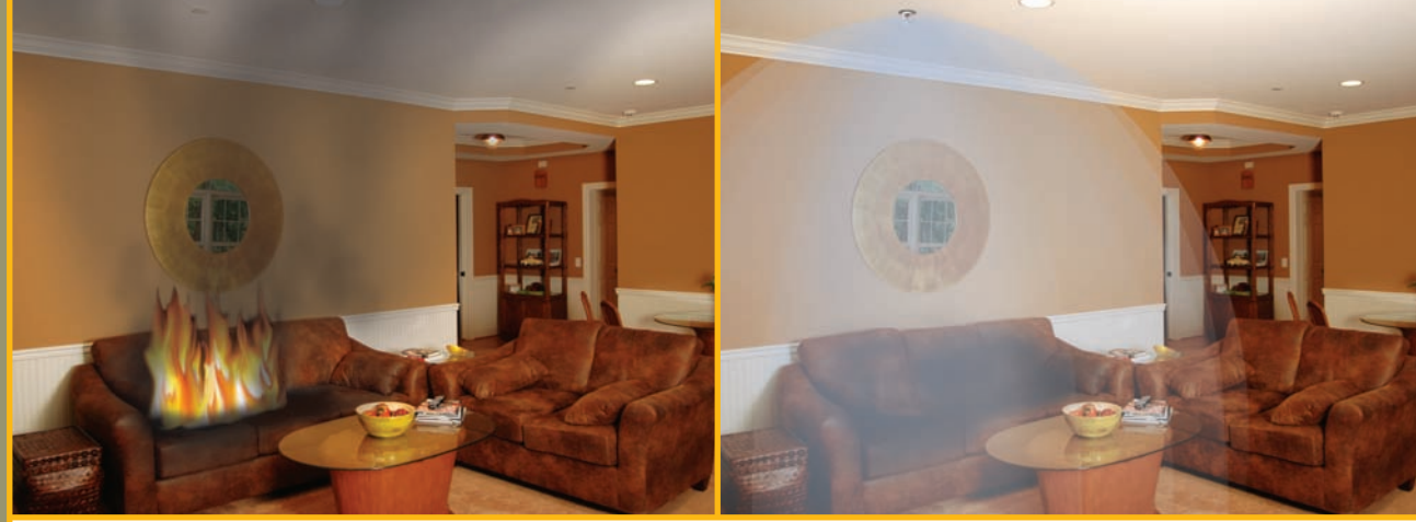
Only the sprinkler closest to the fire will activate, spraying water directly on the fire and the area that the sprinkler has been designed to protect.
