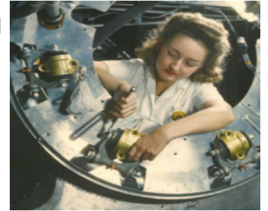
Part of the cowling for one of the motors for a B-25 bomber is assembled in the engine department of North American's [Aviation, Inc.] Inglewood, California,
