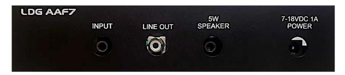
Input: Audio input jack, 3.5 mm (1/8") stereo tip-ring-sleeve jack
