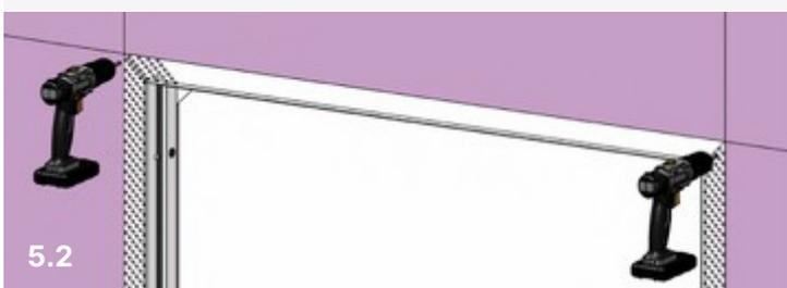
**5.2** Lock the **Frame** into position by adding a fixing to each top corner of the **Fixing Bead**.
