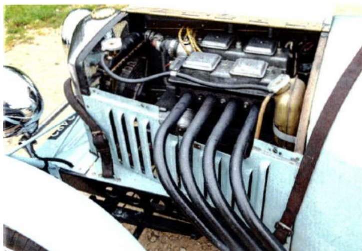
The distinctive twin-cam design of the Riley engine, here in a Nine Brooklands Special, was also powerful and reliable for racing duties.
