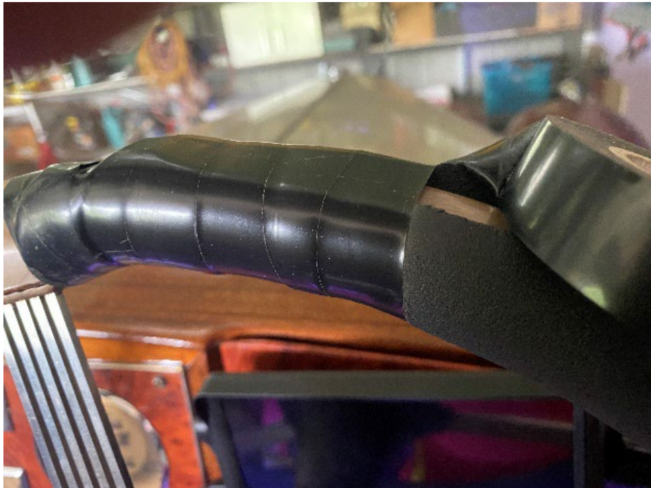
Left: Hot water pipe insulation for padding Right: Binding the insulation with insulation tape
