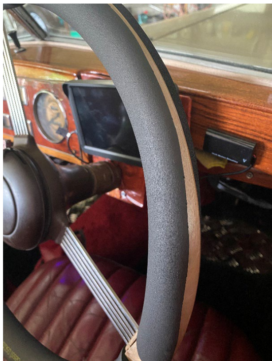
Left: Hot water pipe insulation for padding Right: Binding the insulation with insulation tape
