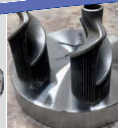
2: Additively manufactured 2-pass mixing element
