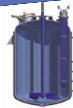
2: 1-stufiger Rührer / single stage agitator
