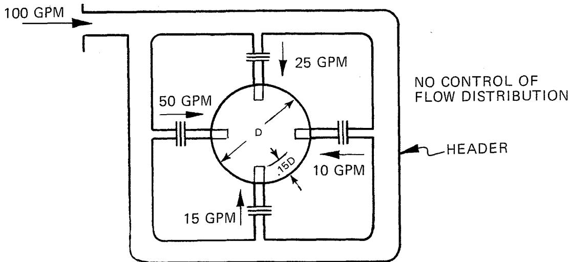
This will occur in headers where the resistance to flow (frictional pressure drop) is so low that there is virtually no change in  $\Delta P$  thru the ports as the flow changes from 50 to 10 GPM.
