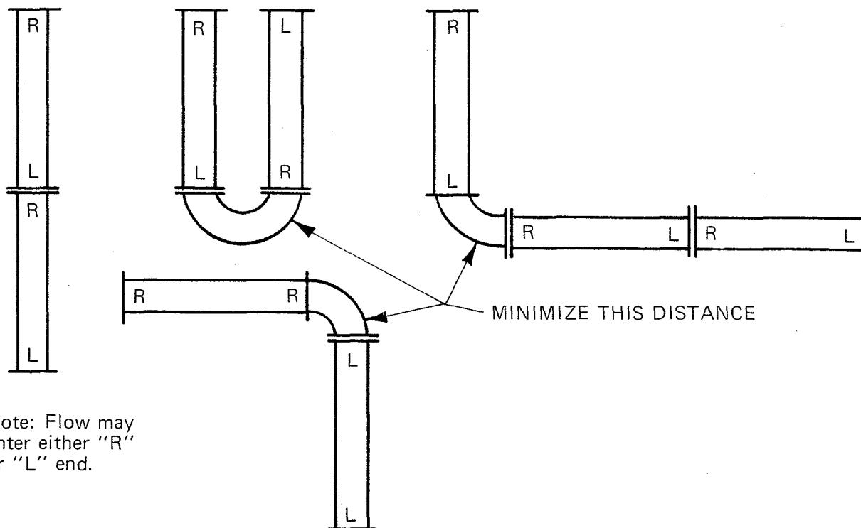
**2.2. DISTANCE BETWEEN MODULES** – The distance between modules should not exceed 2 – 3 pipe diameters.
