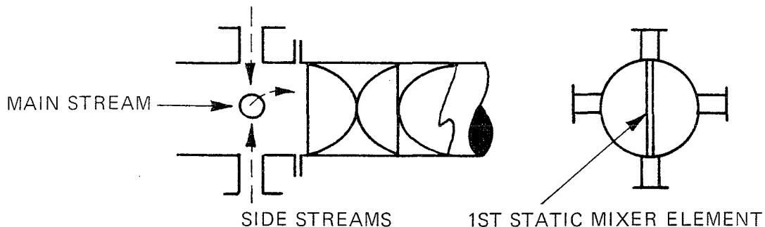
In cases where centerline injection of the minor stream is not feasible, two- or four-point injection of the minor stream is recommended. Flow division of two streams should occur at the first element. Injection velocity should be 2–3 times mainstream velocity, regardless of component viscosities. See Section 4 for recommendations of injection header design.
