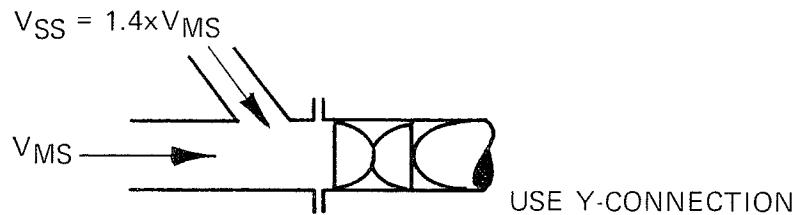
The sidestream velocity should be equal to 1.4 times the mainstream velocity.
