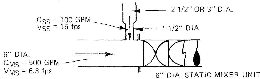
NOTE: To reduce head loss in the sidestream line, the pipe diameter can be reduced to 1-1/2" just prior to the injection point as shown.
