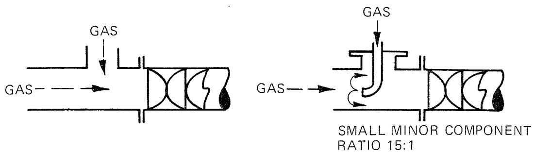
For comparable flow rates, any T-type connection can be used. If the minor component is small, use a nozzle. It is sometimes advantageous to reverse the direction of the minor component to the main flow (As shown in above figure).
