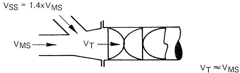
The sidestream velocity should be 1.4 times the mainstream velocity. The injection should occur at an expansion such that the velocity of the total mixture,  $V_T$ , in the expanded pipeline is approximately equal to the initial mainstream velocity,  $V_{MS}$ , in the initial pipeline.
