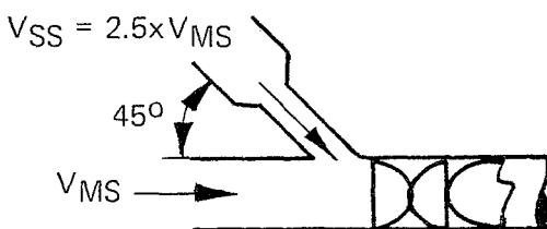
The sidestream velocity should be 2½ times the mainstream velocity.
