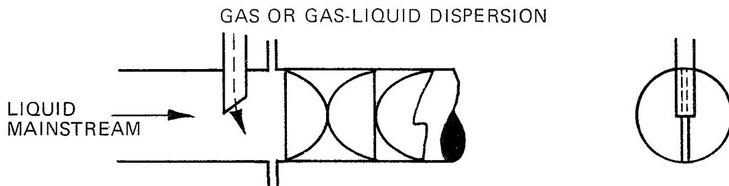
The injection nozzle of the gas should be in the center of the pipe and as close to the first STATIC MIXER element as possible, **less than one pipe diameter**.
