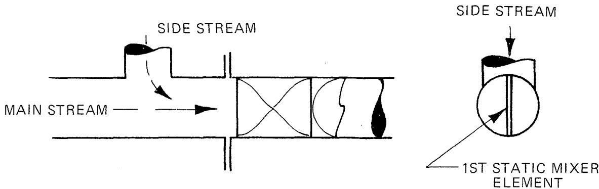
Components may be added by any T- or Y-type connections. The component injection point should be as close as possible to the first element, usually no more than 1 or 2 pipe diameters upstream. The orientation of the T or Y should provide flow division at the first element.
