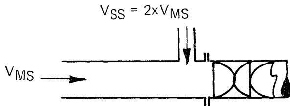
The sidestream velocity should be two times the mainstream velocity.
