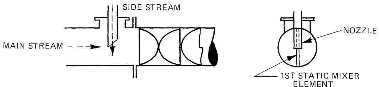
The smaller stream should be injected into the main flow. The injection nozzle of the minor component should be in the center of the pipe and as close to the leading edge of the first element as possible, **less than one pipe diameter**. The smaller stream should have flow division at the first element.
