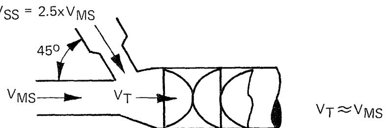
The sidestream velocity should be 2½ times the mainstream velocity. The injection should occur at an expansion such that the velocity of the total mixture,  $V_T$ , in the expanded pipeline is approximately equal to the initial mainstream velocity,  $V_{MS}$ , in the initial pipeline.
