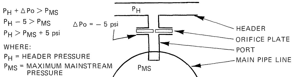
The diameter of the orifice should be sized to provide a pressure drop across the orifice plate,  $\Delta Po$ , of 5 psi at the design flow rate thru each port. If an unequal flow distribution occurs, the port with the greater flow will have a  $\Delta Po > 5$  psi and the port with the lesser flow will have a  $\Delta Po < 5$  psi corresponding to the differential
