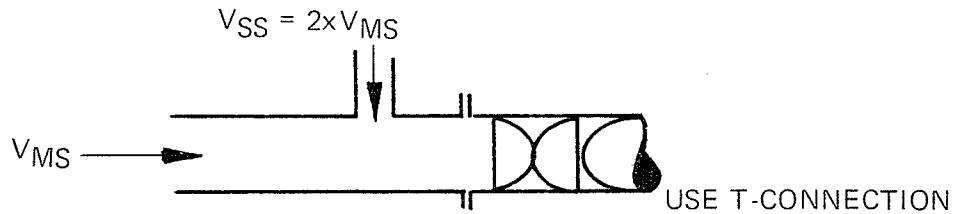
The sidestream velocity should be two times the mainstream velocity.
