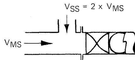
EXAMPLE: Mix 500 GPM of  $H_2O$  with 100 GPM of 25% Sulfuric Acid.
