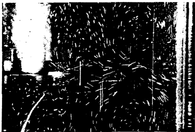
Figure 19—Flow pattern, side view, 4-inch diameter flat blade turbine, 12-inch diameter tank, water. Streak photography showing particle velocities in a 1/4-inch wide vertical plane
