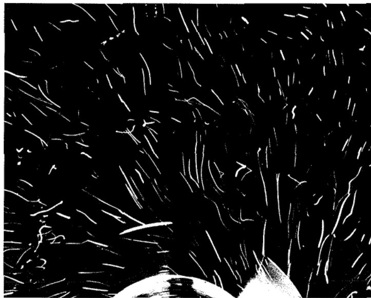
Fig. 4. Typical flow pattern from flat-blade turbine in baffled tank, bottom view, 4-in. diameter turbine, 12-in. diameter tank, water; \frac{1}{4} -in. wide horizontal plane in impeller centerline.
