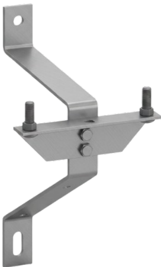
ACAM-SH-12 & ACAM-SH-18: Aluminum single position cutout, arrester, and termination mount. 12 in or 18 in standoff from pole.
