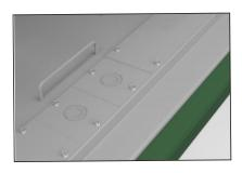
**Step 5.** Remove desired knockout size from wire way knockout plates.
