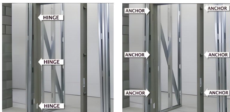
Diagram 1.3 Proper Anchor Spacing
