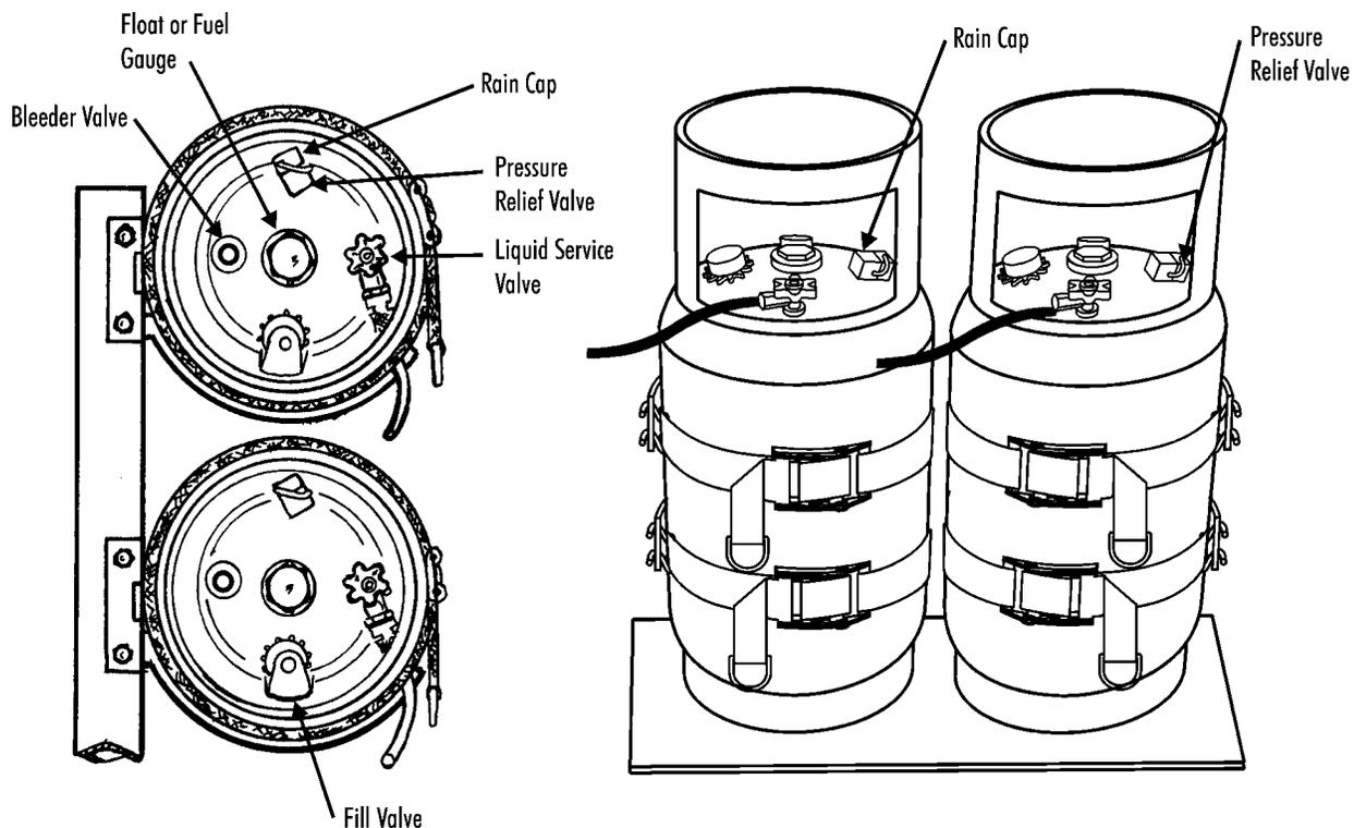
Open the service valve on both tanks and make the appropriate tank selection.
