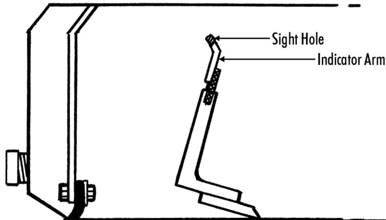
If the sight hole is filled but the blade is too high or low, go to the rear of the conditioner and using a 1 1/8" wrench, first loosen the top nut of the blade level adjusters located on each side of the rear of the conditioner shown below.
