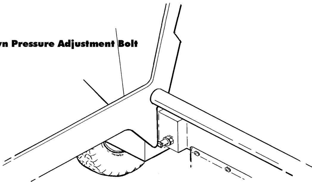
Tighten the bolts against the lift arm and lock with the jam nuts.
