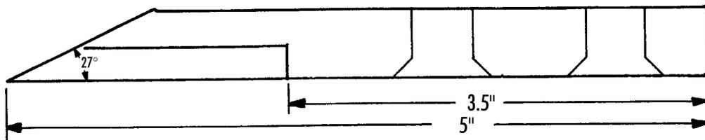
Following the diagrams below, begin to install the blade bolts. Finger tighten the bolts. **DO NOT** use lockwashers as they will damage the blade holder. There are two ways of properly tightening the blade bolts:
