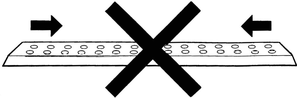
The blade holder is feathered 1/16" over the last 7" on each end. This prevents ridges forming on the ice during the resurfacing operation.
