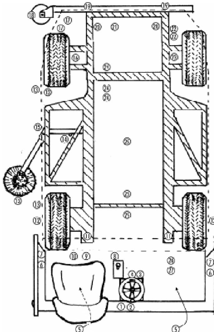
Using the drawing on the adjacent page as a guide. Make sure you grease all 25 lube points as follows:
