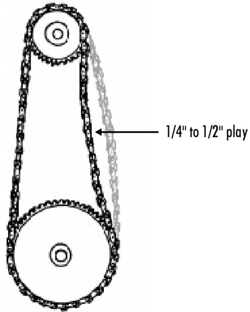
To adjust the chain tension, loosen the motor mount plate bolts and slide the motor mount until you get the proper tension, then re-tighten the motor mount plate bolts.
