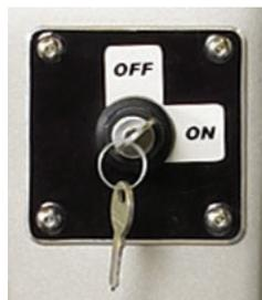
Turn the ignition key to the right or ON position to switch on the ice resurfacer and put it into operation.
