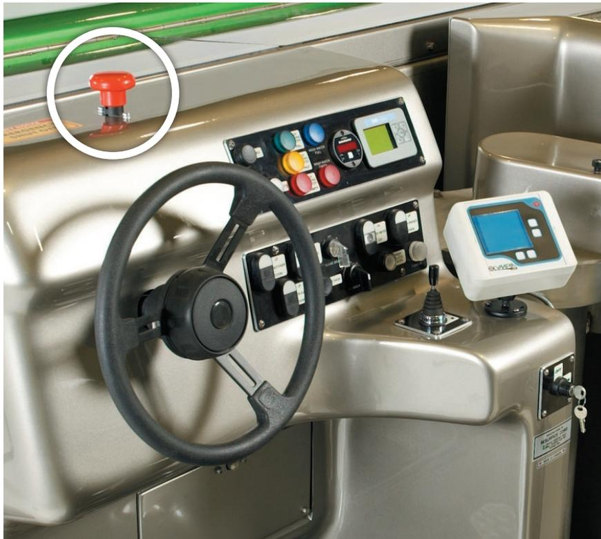
Fig. 1.1: Emergency Shut off switch on the OLYMPIA
