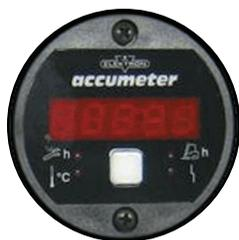
The accumeter is equipped with a digital LCD display. This will display the remaining capacity of the batteries. By pushing the white button it will change to operating hours. By pushing the white button a second time it will display hours until the next service is needed. A third push of the button will display operating temperature. A slashing red light in the right corner will indicate low electrolyte level.
