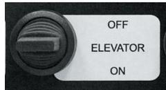
Turn both augers ON (horizontal and vertical auger), by pushing the switch down. Turn both augers OFF by lifting the switch to the off position.
