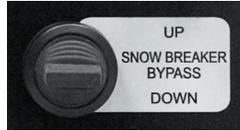
Is a backup system which allows for the manual operation of the snowbreaker.
