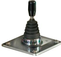
Unless moving the ice resurfacer, always make sure the gear shift selector is in the neutral position. To move the ice resurfacer forward move the gear shift selector to the forward position. To reverse the ice resurfacer, move the gear shift selector to the reverse position.
