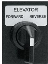
Left switch position: Snow is transported from the conditioner into the snow bin by the horizontal and vertical augers
