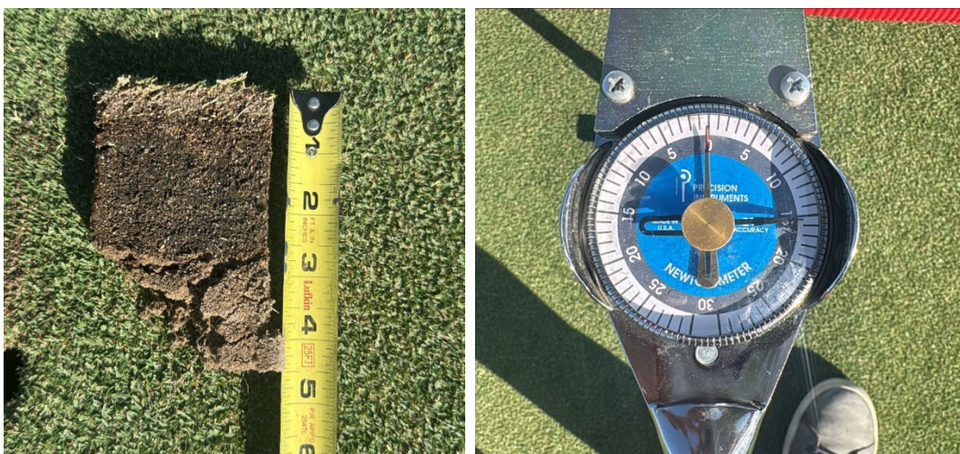
Left: Roots are healthy in greens and extend to over 4 inches. Right: The shear strength numbers were good, with values ranging from 15 to 17 Nm.
